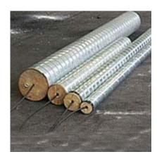
Canistered anodes are primarily designed for special applications such as wet, marshy areas or soil conditions where caving is likely to occur. Benefits such as reduced installation costs and convenience of handling make the canister attractive for standard applications also.
