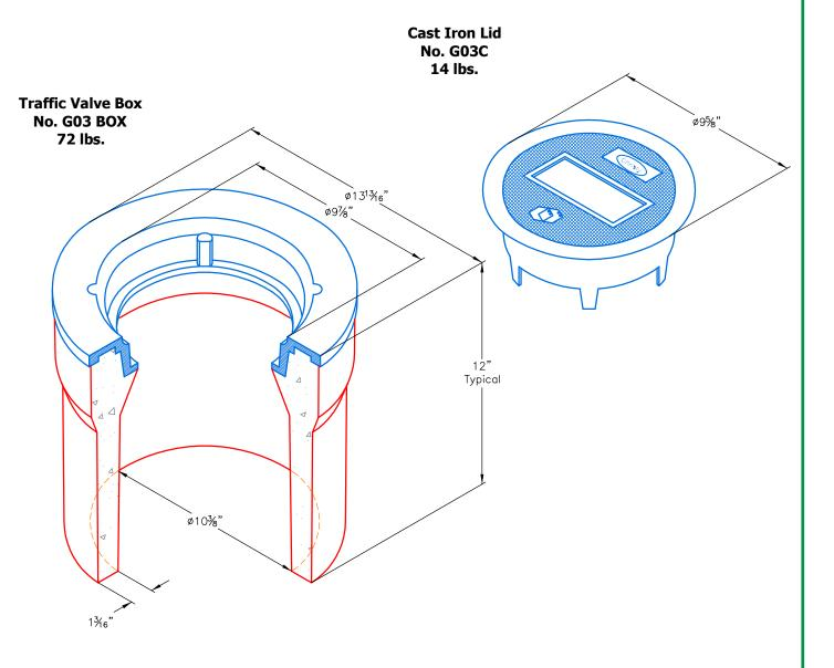
A high density reinforced concrete box with cast iron ring for heavy traffic areas. Engineered and designed to be interchangeable with the Brooks 3RT. Approximate dimensions and weight shown.
