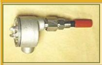
The GMC STAPERM™ thru-hull mounting assembly is designed to provide easy installation of special submersible STAPERM™ reference electrodes. Each electrode comes complete with a test lead junction box, electrode sealing system and 3/4" NPT threaded fitting for mounting directly through the structure wall. The electrode can be readily removed and reinstalled from the exterior of the vessel (not under pressure).
