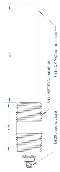
Model FS-xxx-SW - Short Wire termination is 1 foot of #16 AWG lead wire Model FS-xxx-LWnnn - Long Wire termination is nnn feet of #16 AWG lead wire
