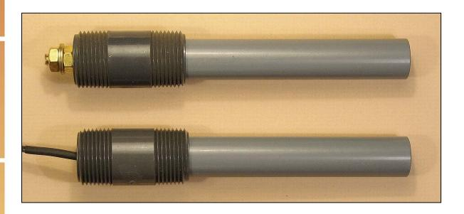
**Model FS,** with a CPVC extension tube and a ¾ inch NPS PVC nipple, is designed for standard duty applications. It can be used at pressures up to 40 psi (270 kPa) and intermittent temperatures up to 180°F (82°C). For applications involving pressures up to 75 psi (0.5 MPa), our Heavy Duty Through-wall Reference Electrode, Model FH, is preferred.
