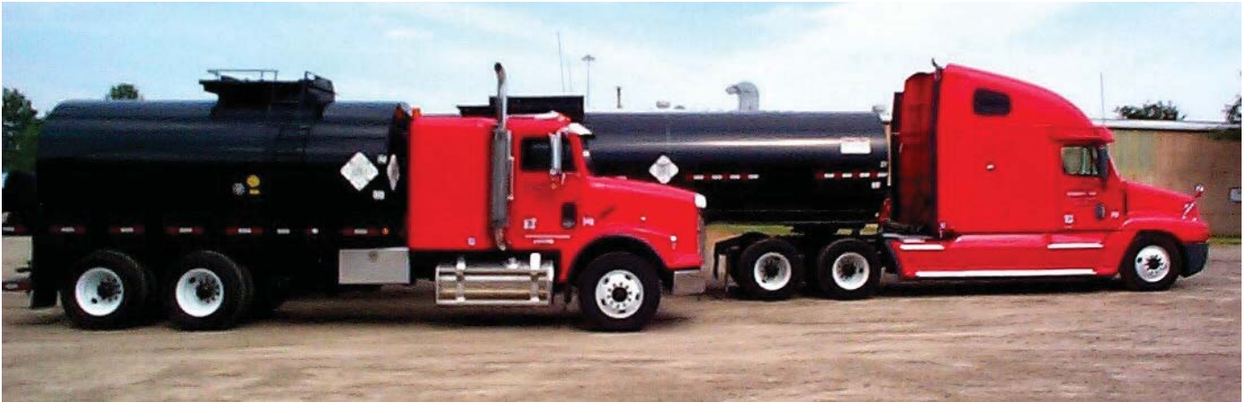
Fill-Coat #1 is delivered to the job site via Trenton's 3000- and 6000-gallon tank trucks that are heated and insulated.
