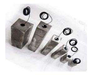
Electrolytic conditions in the soil surrounding a buried structure determine the type of anodes employed in a cathodic protection system. In low-resistivity soil (under 2,000 ohm-cm), MESA's line of magnesium anodes are the most economical choice. H-1 anodes are cast to meet ASTM B843, Alloy AZ63.
