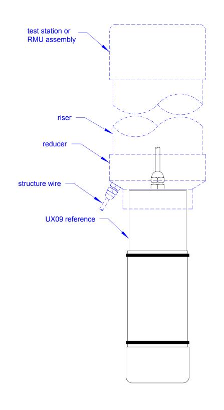
Typical installation of Model UX09 reference electrode on an RMU or test station riser. Components shown in dashed lines are user supplied.
