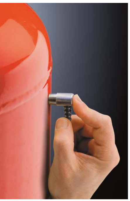
UTG M Multiple Echo Thru-Paint probe measures the thickness of a painted structure without having to remove the coating.
